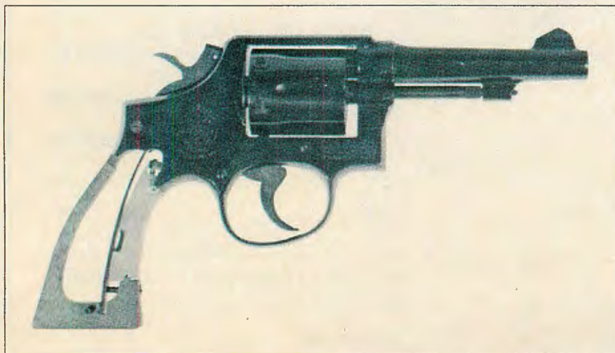
Below: With grips removed, cuts in frame can be seen where alloy insert replaces part of front strap.
